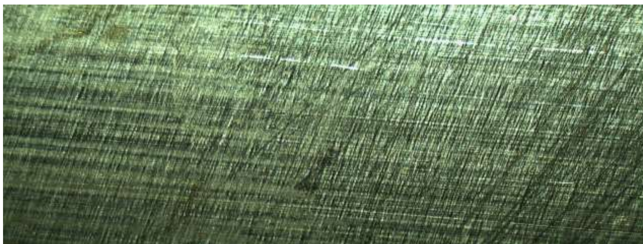
Photo № 5 - Presence of multiple scratches along the metal blade – stereomicroscopy
